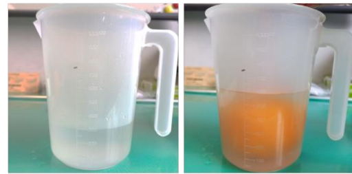
Figure 2. Measuring volume using Archimedes approach
