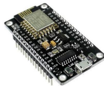
Gambar 3. NodeMCU ESP8266 Lolin
