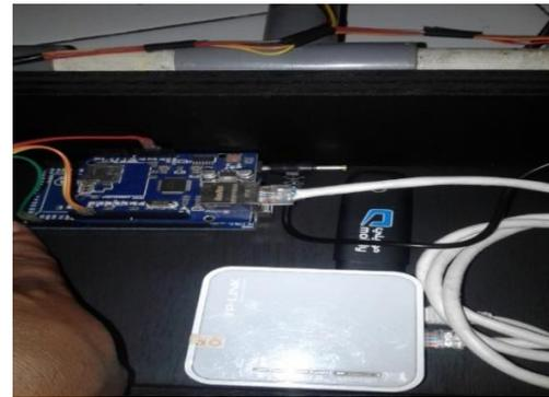
Gambar 6. konfigurasi Modem Huawei E3372, Router TP-Link TL-MR3020 ke ethernet shield
