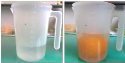
Figure 2. Measuring volume using Archimedes approach
